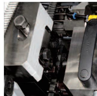
▲ New arrangement of the pressure jaws also for production of D-head and offset nails
